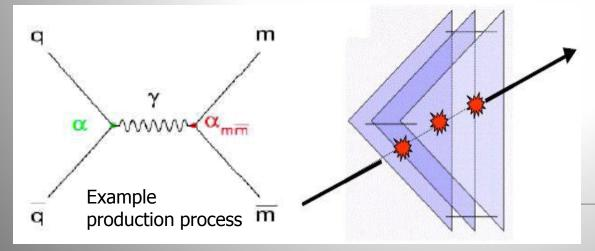
Monopoles will 'burn' through the plastic sheets of the experiment or get trapped in the dense material of the trapping detector
