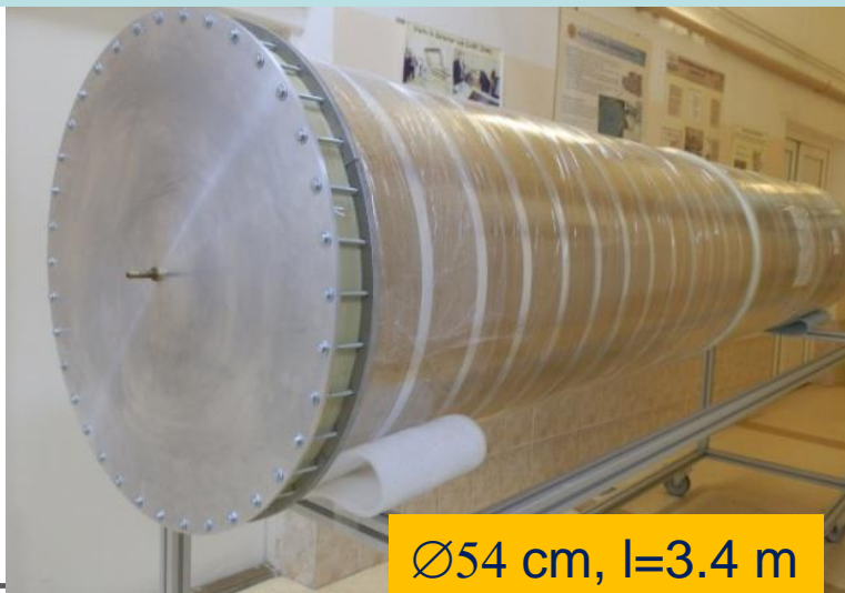
Cylinder C2, preparation for vacuum tests
