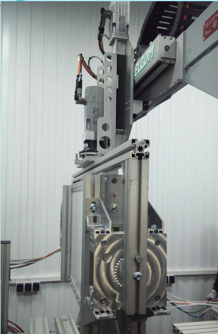
MRPC prototype in positioning device
