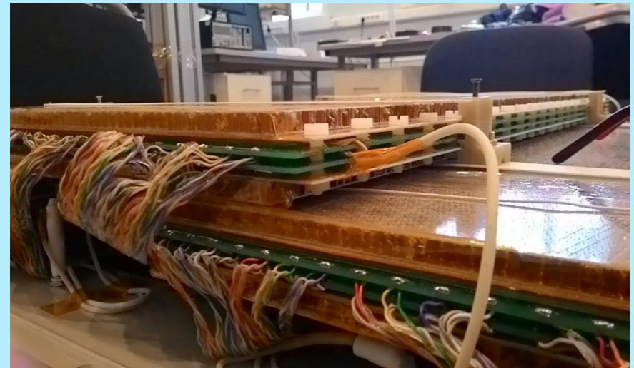
Assembled triple-stack prototypes in module
