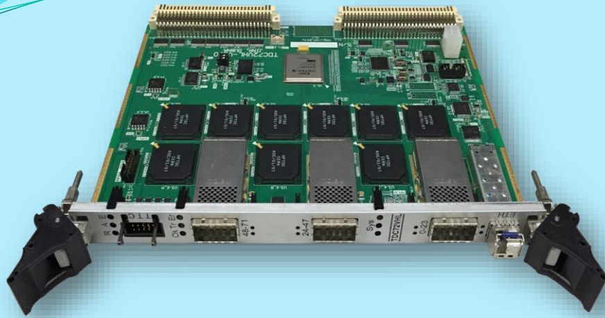
TDC72VHL with CPX(InfiniBand) connector
