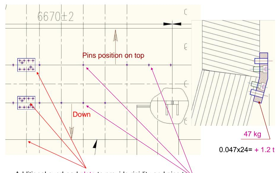
Additional overhead plate to provide rigidity and pins to weight transfer plates from the stove to the plate. The pins run on collapse: Square contact 3.3x8 x 10 = 240 cm2, the permissible load on the crushing 384 tons, Less far as possible from the 6 plates (18.5x6 = 111 tonnes).
