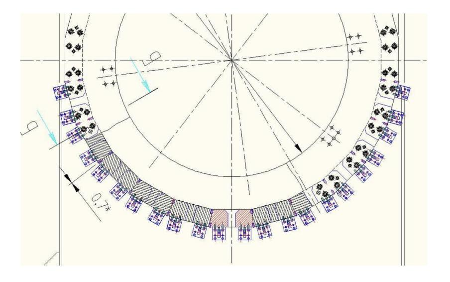
Material for pins: steel 40X (Shear stress - 1850 kg / cm2). Cross-sectional area 8.5 cm2, load capacity 15.8 tonnes. The total shear strength on one cradle 632 tons.
