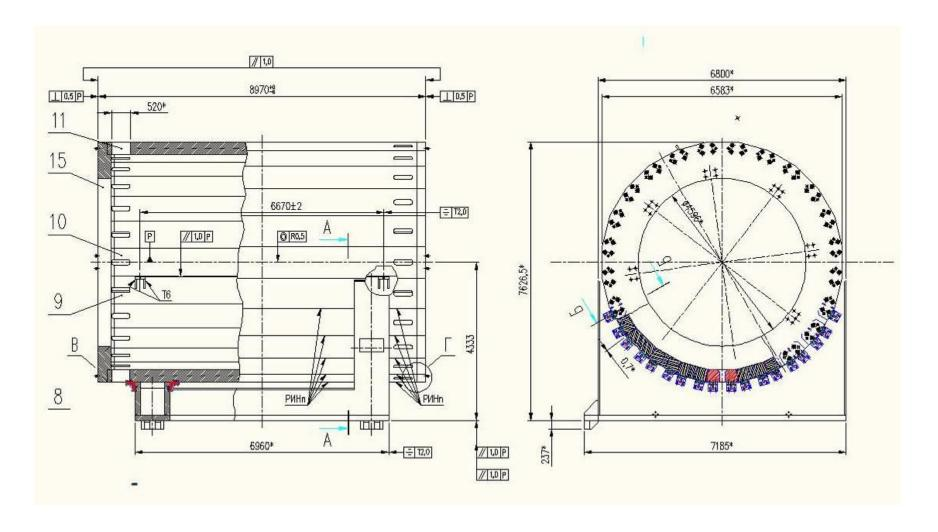
Fixing the lower plate 11 to the lodgement (cradle) through the brackets (22\*4 = 88 pcs.) by means of bolts M30 class 10.9 and pin diameter 33 mm (interference fit H7 / p6)
