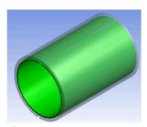
The LTS shield is a multilayer unclosed winding made of the superconducting foil.
