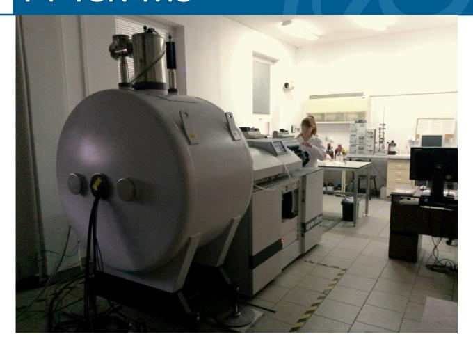
Fourier Transform Ion Cyclotron Resonance Mass Spectrometer
