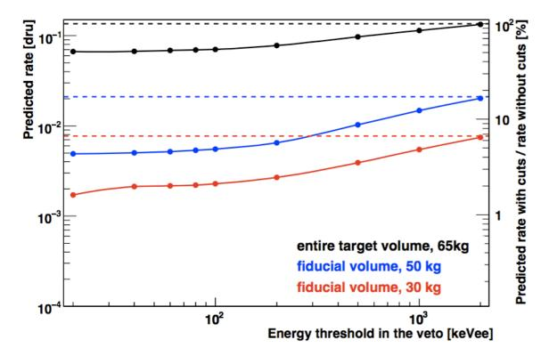
Fiducial volume and active veto cuts: up to 95-99% efficiency for electron recoil background rate reduction
