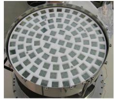
80 PMTs on the bottom, 98 PMT in the top array, 64 PMTs in the active veto
