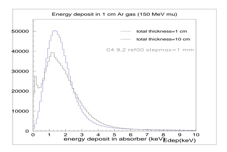
The reason of the strange behaviour is the so called width correction algorithm in the fluct. model. In this algorithm the energy fluctuation for a given step can depend on the energy deposit values in the preceding steps. Introducing a different width correction algorithm -where the correction depends on the actual energy deposit only- cures this anomalous behaviour.
