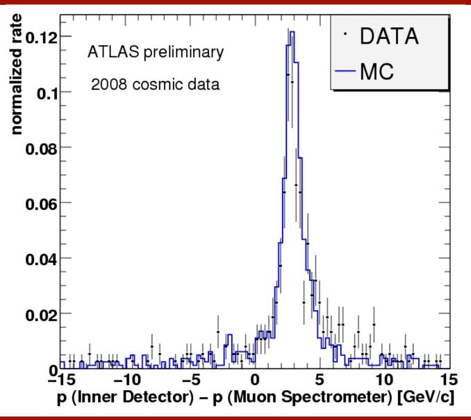
Cosmic ray energy loss in the calorimeters
