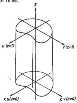
G4SurfaceOfLinearExtrusion (const &G4Curve curve, G4double length)
