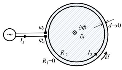
energizing current in the outer ring:  $I_1(t) = \alpha t$
