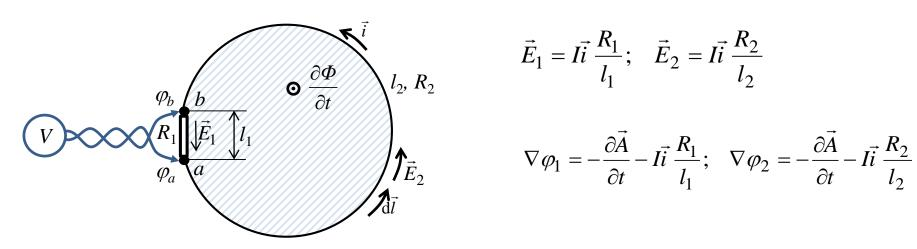
$$\vec{E}_1 = I\vec{i} \frac{R_1}{l_1}; \quad \vec{E}_2 = I\vec{i} \frac{R_2}{l_2}$$
