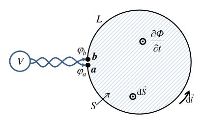
$$\int_{a}^{b} \vec{E} \cdot d\vec{l} = \int_{a}^{b} \left( -\frac{\partial \vec{A}}{\partial t} - \nabla \varphi \right) \cdot d\vec{l}$$
