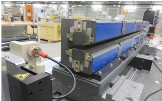
Magnetic measurements of full DL & final field tuning
