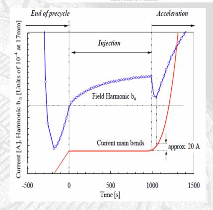
Need to keep both b<sub>3</sub> and its drift below 1 unit
