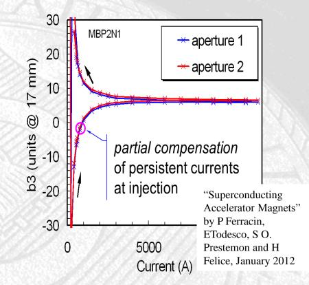
The above process leads to a partial compensation of the error fields at injection, a (hopefully small) negative value usually dominated by the sextupole component, b3.
