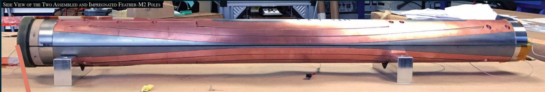
SIDE VIEW OF THE TWO ASSEMBLED AND IMPREGNATED FEATHER-M2 POLES
