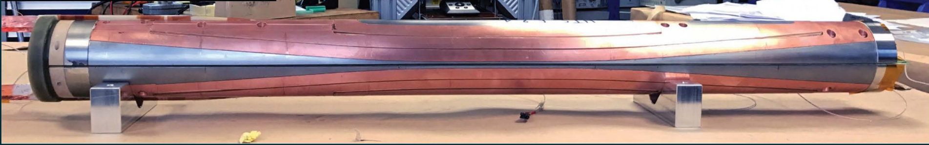
SIDE VIEW OF THE TWO ASSEMBLED AND IMPREGNATED FEATHER-M2 POLES
