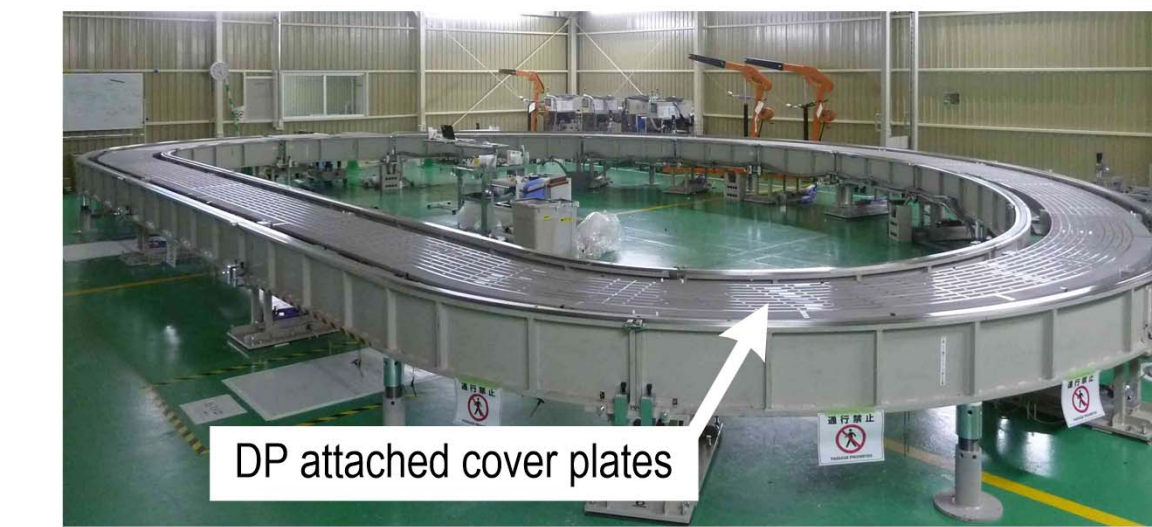
b) DP inserted conductor into RP groove and attached cover plates
