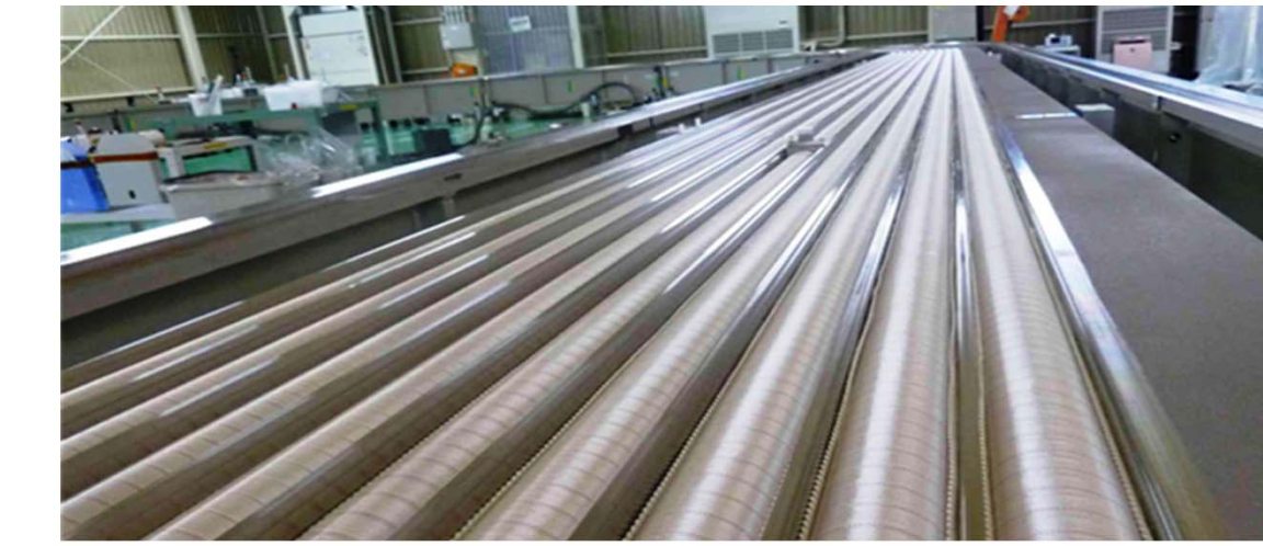
a) Insulated conductor inserted into RP groove
