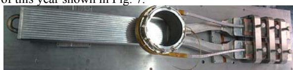
Fig.6. Tested joint sample connected to transformer
