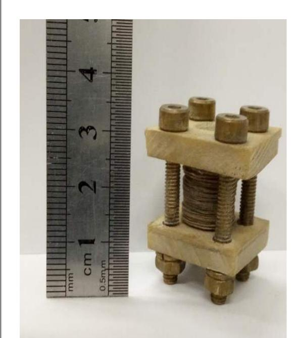
The HTS magnet is composed of 80 REBCO annular plates, including 40 silver-plated REBCO annular plates and 40 copper-plated REBCO annular plates, inserted insulating polypropylene laminated paper (PPLP) between adjacent REBCO annular plates.
