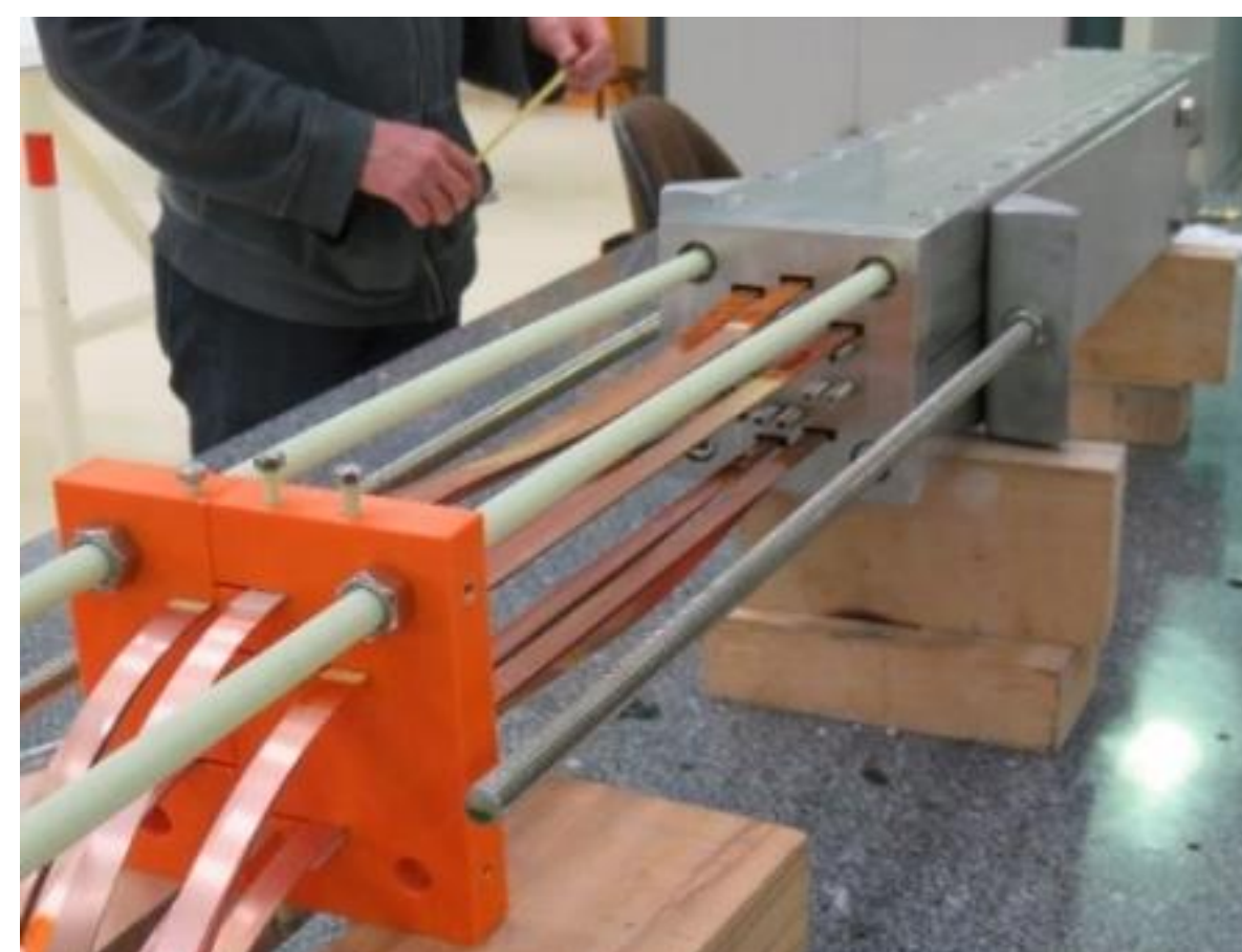
Demountable inter-coil connections: 160-mm long SnIn splices
