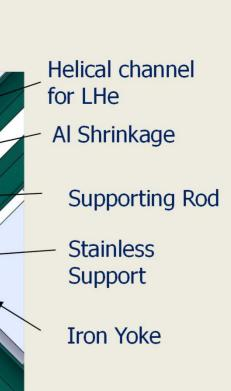
The challenging most specification to meet is the low thermal losses allowed for the magnet, so its design was aimed at optimizing this requirement.
