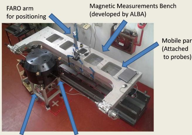
Hall probes (3-axes) Cyclotron Magnet
