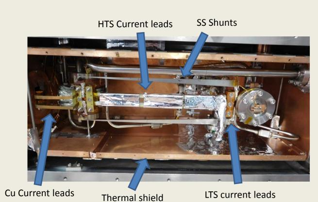
High thermal efficiency connection box was developed: - HTS current leads anchored to refrigeration cryogens at two different temperatures.
