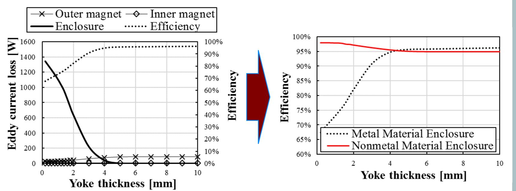
At the yoke thickness of 1.2 mm suggested in this study, there were no changes in the permanent magnet eddy current loss or the iron core loss, but a greater loss occurred in the enclosure.
