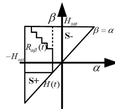
Fig.2. The modified hysteresis operator ( $H_{sat}$  is the saturated magnetic field intensity).
