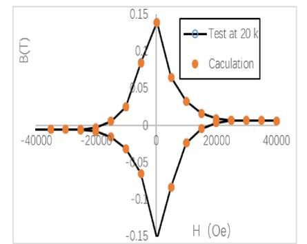
Fig.3. Result comparisons of MgB<sub>2</sub> hysteresis loop at 20 k based on test and calculation
