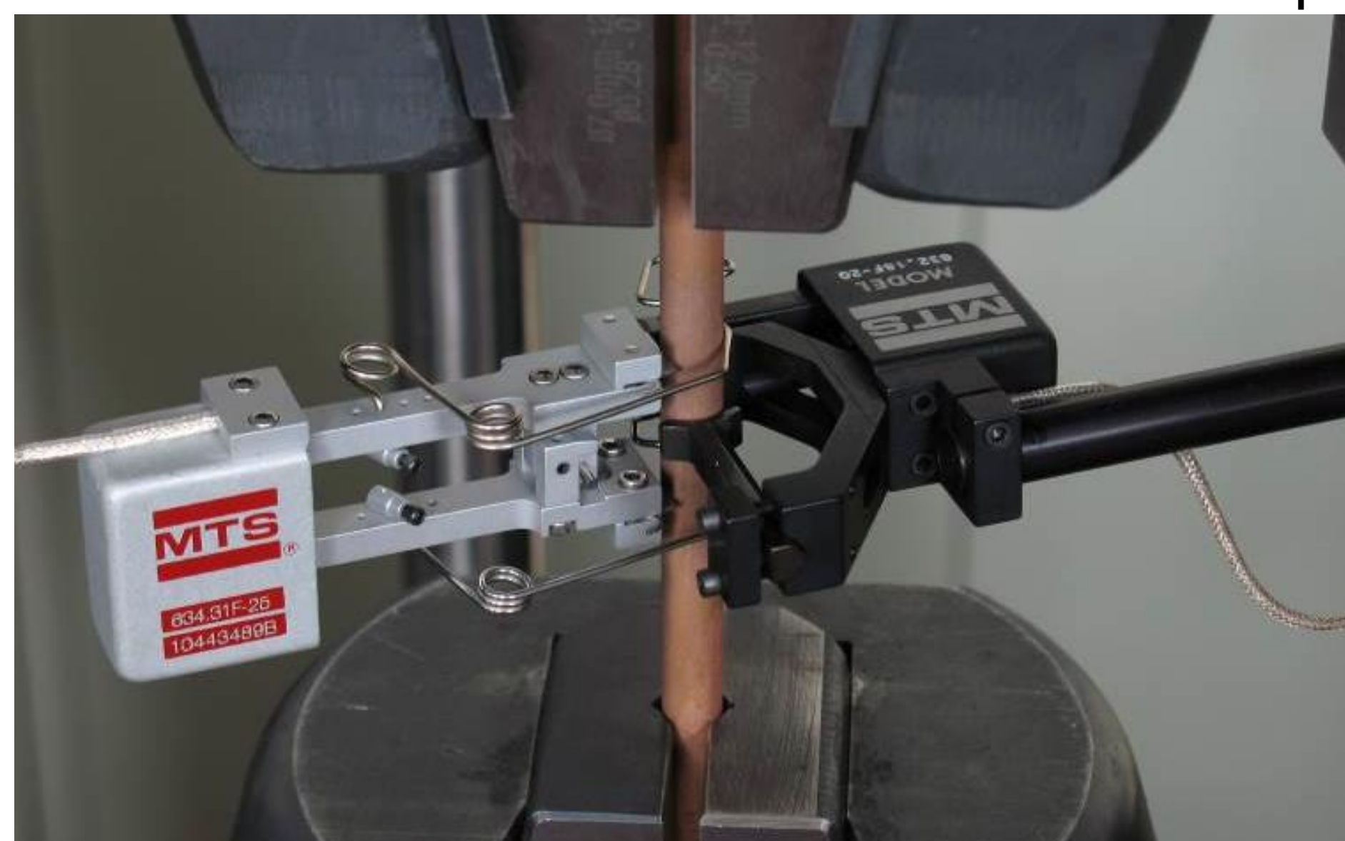
Fig. 8: Set-up with extensometers for axial and for radial strain measurement.
