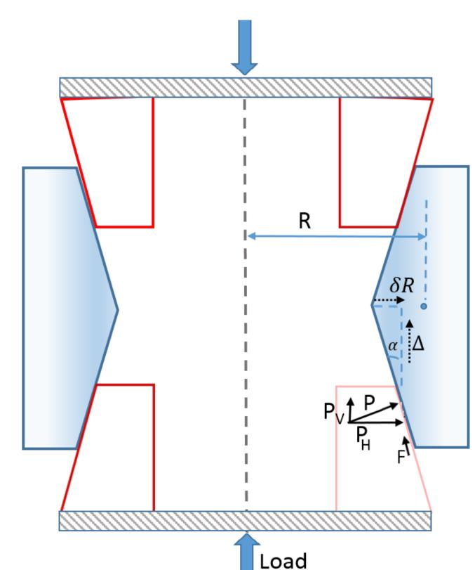
Assuming the spring is being compressed, the total radial force acting on the outer ring will be equal to:
