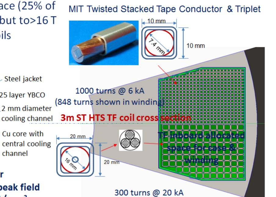
(204 turns for full winding; additional turns needed)
