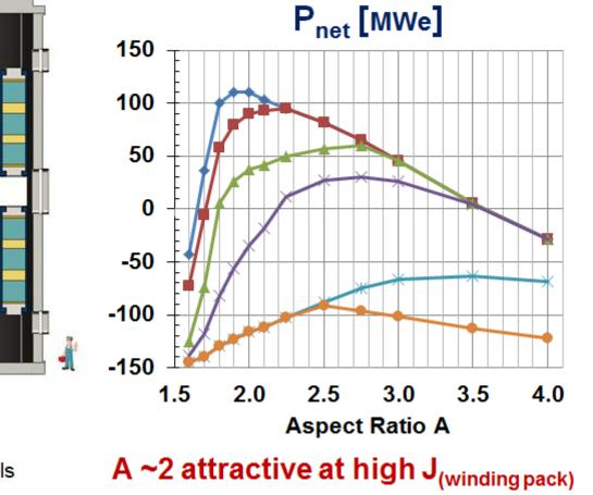
major radius R<sub>0</sub>=3m, heating power P<sub>NNBI</sub>= 50 MW
