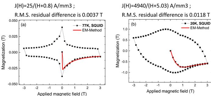
Fig. 1. The magnetization of sample was measured by SQUID under 77K and 20K. The black dots mark the measurement result, and the red line shows the calculations by EM-Method.
