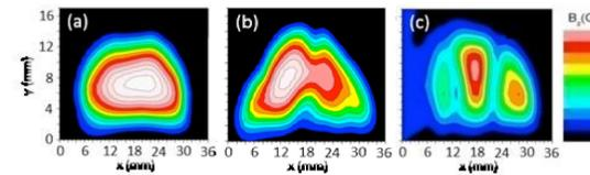
Fig.4. Three different half bulks magnetized by Field-Cooling process under 77K were measured by Hall probe system. The magnetic field normal to the surface is shown.
