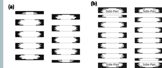
Fig.5. (a) Diagram of current penetration of a BHTSU with 10 bulks magnetizing by Field-Cooling with 1 Tesla and with J(H) curve in Fig.1(b) adopted. (b) Side-Pair added.
