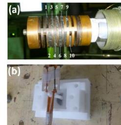
Fig. 3. (a) A BHTSU with 10 half bulks, conducting to a cryocooler, can be cooled down to 7K. (b) A half bulk, magnetized and immersed in LN2, is under 2D scanning by Hall probe.
