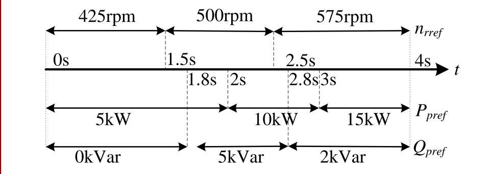
In the simulation process, the brushless doubly fed generator is operated at sub-synchronous, synchronous and super-synchronous speed respectively. Active and reactive powers are given a step change in different moments.
