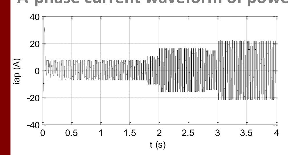
Both active and reactive power vary with the given value. The power winding current is in good sinusoidal shape, and the frequency remains constant at 50HZ when the speed, active or reactive power is changed.
