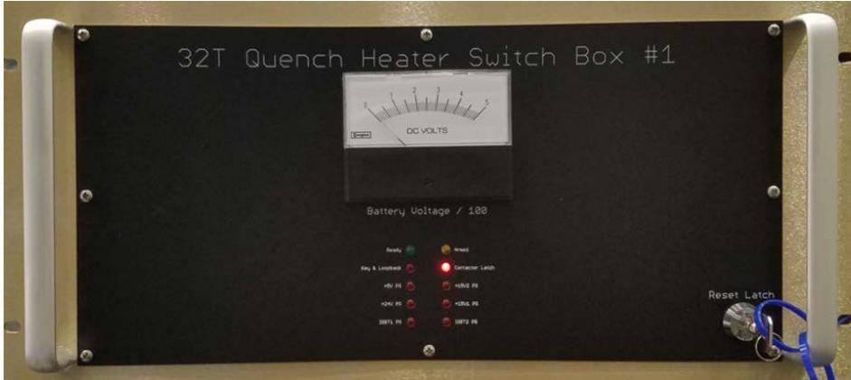
Battery Bank has a peak possible current of 1600 A and the switch boxes must be able to break it
