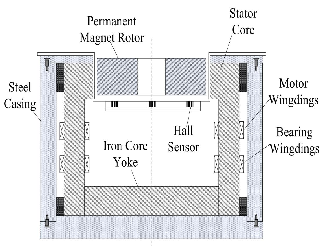
The stator of the motor is distributed evenly around the rotor with six L-shaped iron core legs. Each of the motor windings and bearing windings of the BPMSM, whose numbers of pole pairs are  $P_M=1$  and  $P_B=2$ , respectively, has six concentrated coils distributed on the iron core leg.
