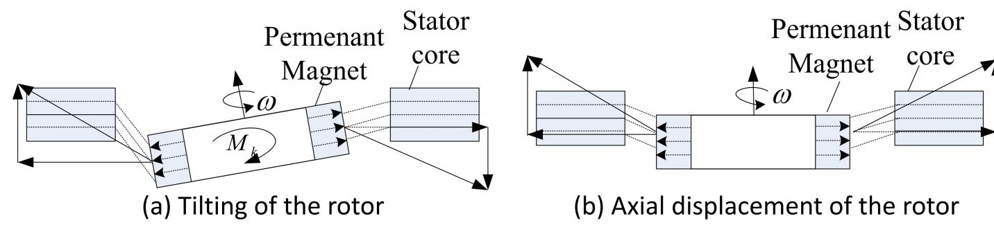
The PM rotor is passively stabilized by reluctance force in the axial and tilting directions.
