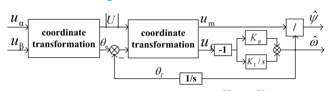
Closed-loop transfer function:  $g(s) = \frac{K_P s + K_I}{s^2 + K_P s + K_I}$
