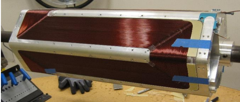
Closed-loop-coil with Cu wire finished on the winding fixture
