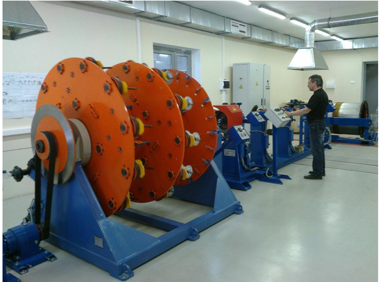
Machine for production Nuclotron-type superconducting cable
