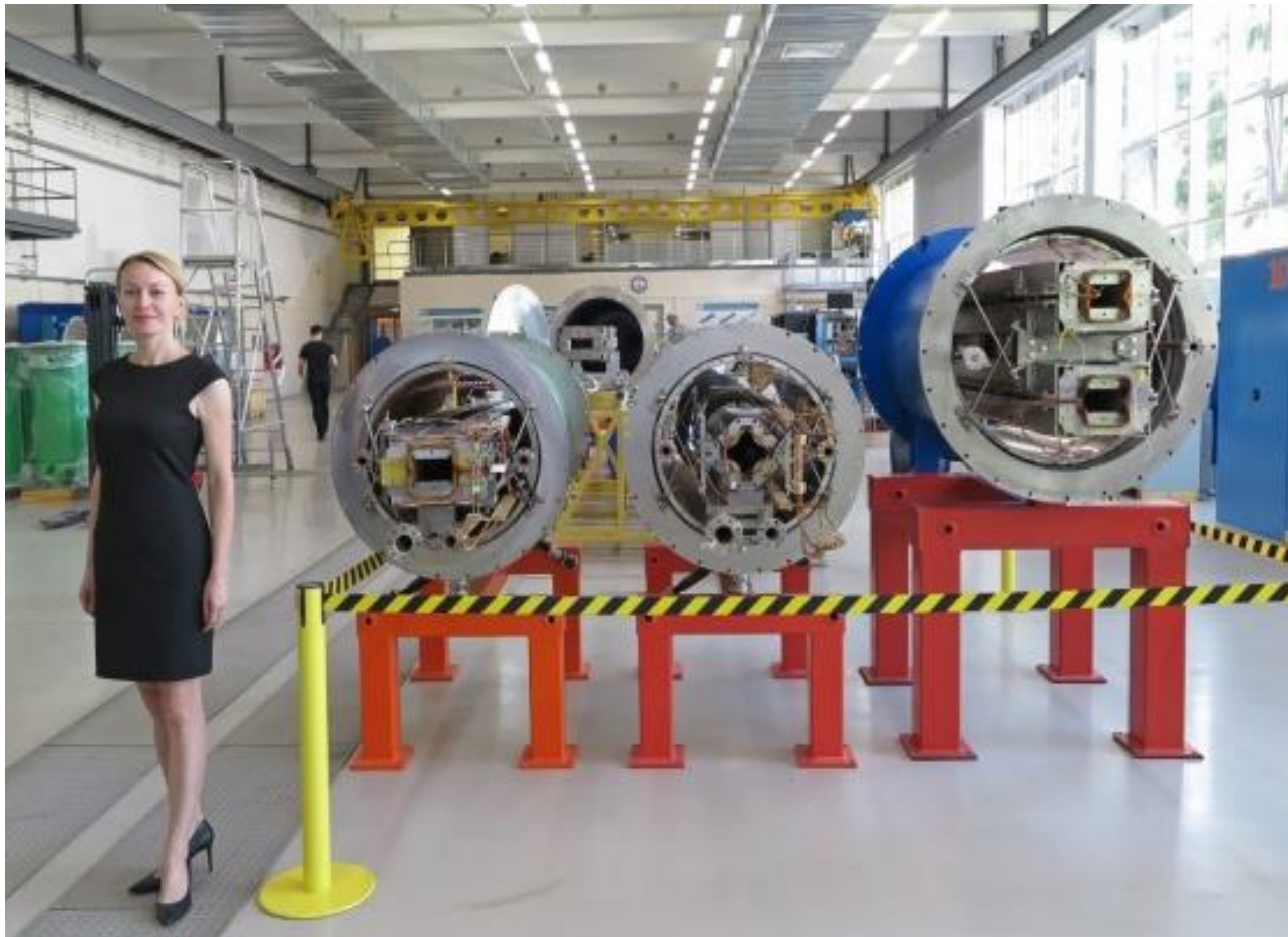
Series dipole magnet (left) and doublet (center) for NICA booster, and pre series dipole magnet for NICA collider (right).
