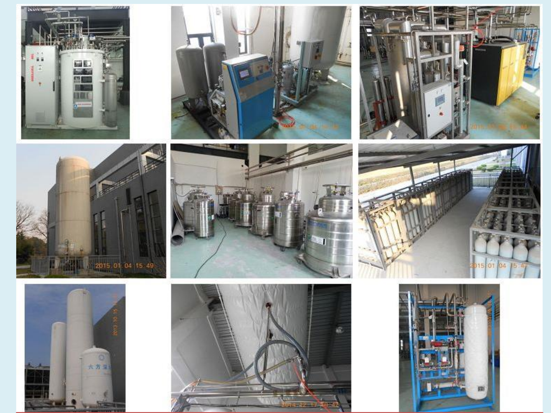
LHe plant (360W at 4.5 K or 110 L/h has been operated LHe production for 5 years)
