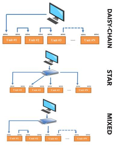
**Paralleling** is also performed using the SFP+.
