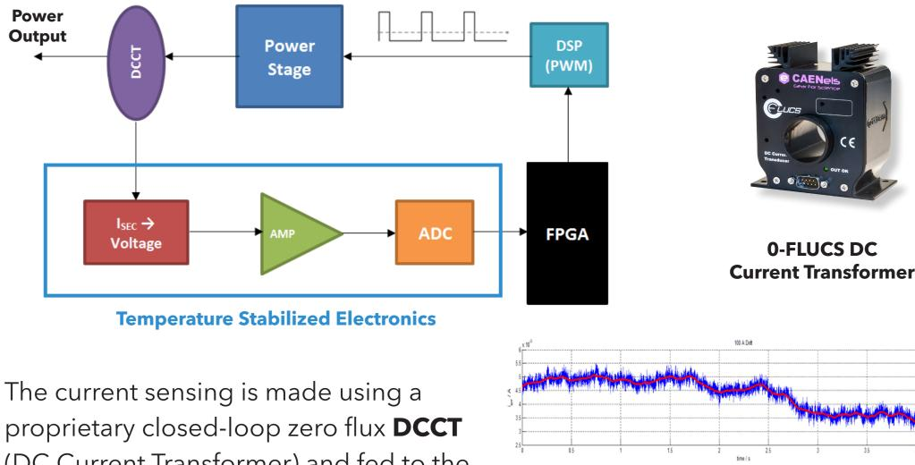
The current sensing is made using a proprietary closed-loop zero flux **DCCT** (DC Current Transformer) and fed to the ADC via a temperature-stabilized signal conditioning section to reach a **TC < 1 ppm/°C**.
