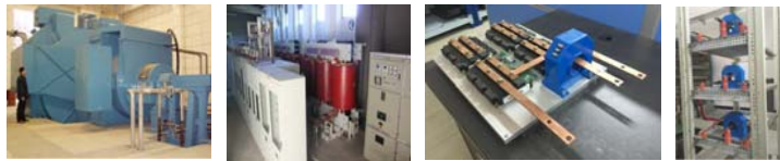
Fig. 5. Photos of facilities and prototype of inverters of active regulator. (a) Pulse generator. (b) Rectifiers. (c) Single H-bridge inverter. (d) Cascade H-bridge inverters.
