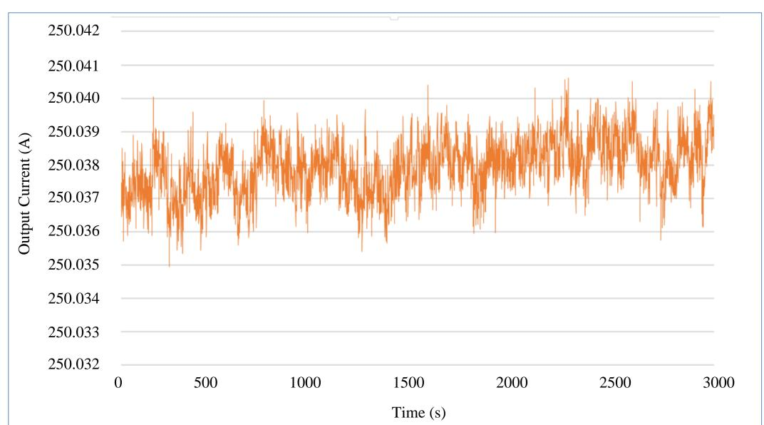
Experiment result of output current long term (up of 8 hours) performance. The main power supply output current within  $\pm 0.005A$  or within  $\pm 20$  ppm. The long term performance of the proposal main power supply is better than it specified  $\pm 50$  ppm range.
