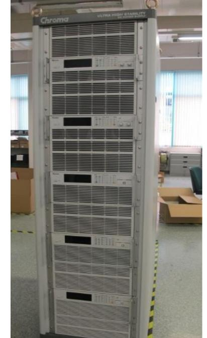
A power rack size is 19 inch, The space of dimensions (H\*W\*D) is 2030mm\* 600mm\* 900mm.
