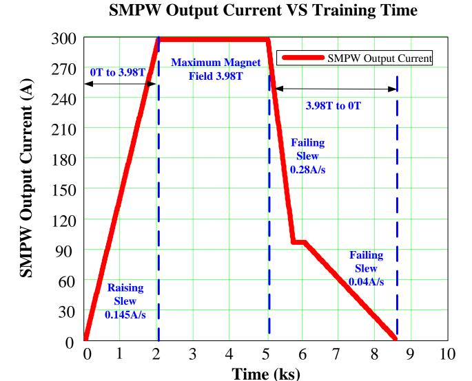
Step 1: SMPW output current from 0A to 297A, SMPW was reached maximum field of 3.98 Tesla and keep the output current to observe the magnetic field and current stability.
