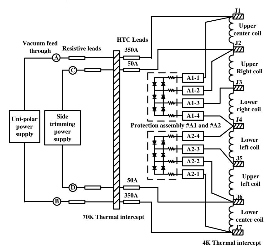
The electrical layout of SWLS, the main power supply is responsible for charging the main coils to eliminate the first and / or second field integral.
