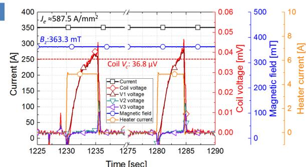
Figure 5 (b). Enlarged voltage and heater current pattern of the Cu strip inserted MC-NI coil during 2nd and 3rd quench.
