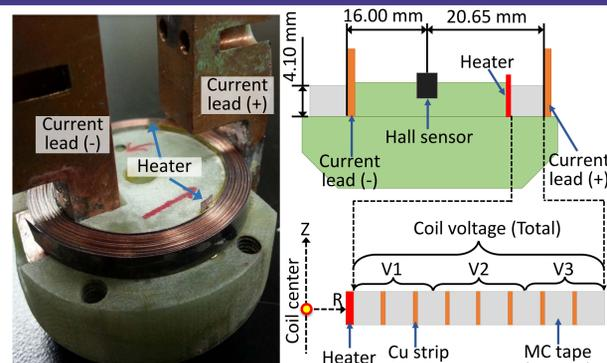
Figure 2. No-insulation test coil wound with metallic cladding REBCO tape. A total of 7 Cu strips were inserted and equally distributed within the winding.
