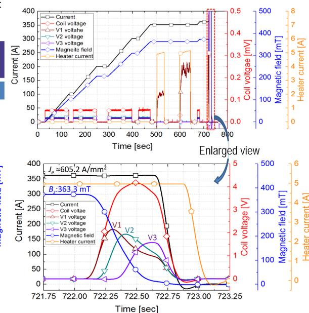
Figure 6. Quench propagation result of the Cu strip inserted MC-NI coil during the thermal runaway quench test.
