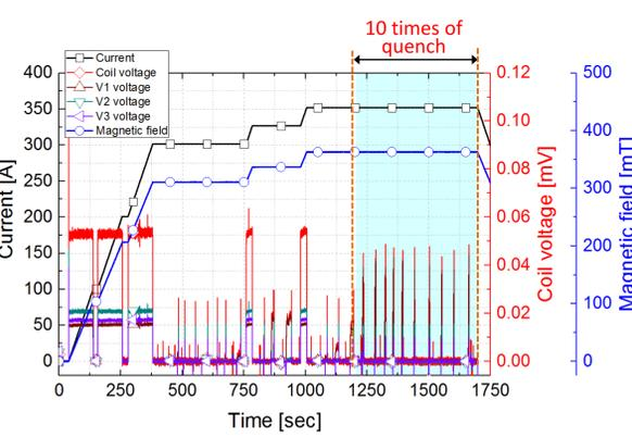
Figure 5 (a). Whole operating procedure of the Cu strip inserted MC-NI coil during the multiple quench test in a bath of liquid helium at 4.2 K.
