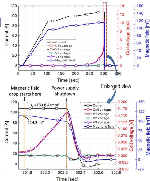
Figure 3. Voltage and magnetic field vs. time curves of the Cu strip inserted MC-NI coil during the over current quench test in a bath of liquid nitrogen at 77 K.
