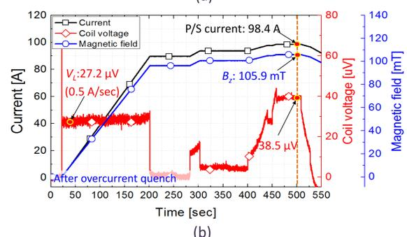
Figure 4.  $I_c$  measurement results of the Cu strip inserted MC-NI coil: (a) Before overcurrent quench, (b) After overcurrent quench.
