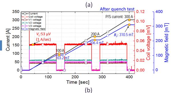
Figure 7. Step charging results of the Cu strip inserted MC-NI coil: (a) Before both quench test, (b) After both quench test.
