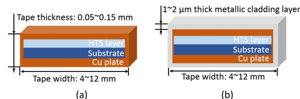
Figure 1. Conceptual comparison between NI and MC REBCO tapes: (a) No-insulation REBCO tape, (b) Metallic cladding tape.
