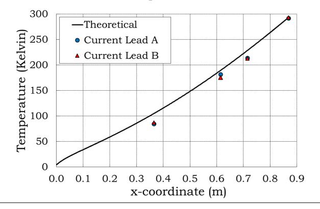
Conclusion. A pair of brass current leads for the Iseult/NeuroSpin project have been designed and tested at Saclay The measurements have shown a good agreement with the calculations; the helium mass flow required is of 0.095 g/s at 1 483A corresponding to a 1.23 W/kA ratio. A small and inconsequential discrepancy has been measured between leads which nevertheless fulfill the specifications, notably in case of lack of helium cooling.
