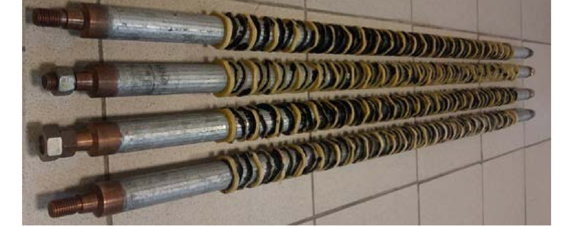
Fiber-glass double-threaded spiral guide (to elongate gas trajectory and thus improve cooling conditions by helium gas).
