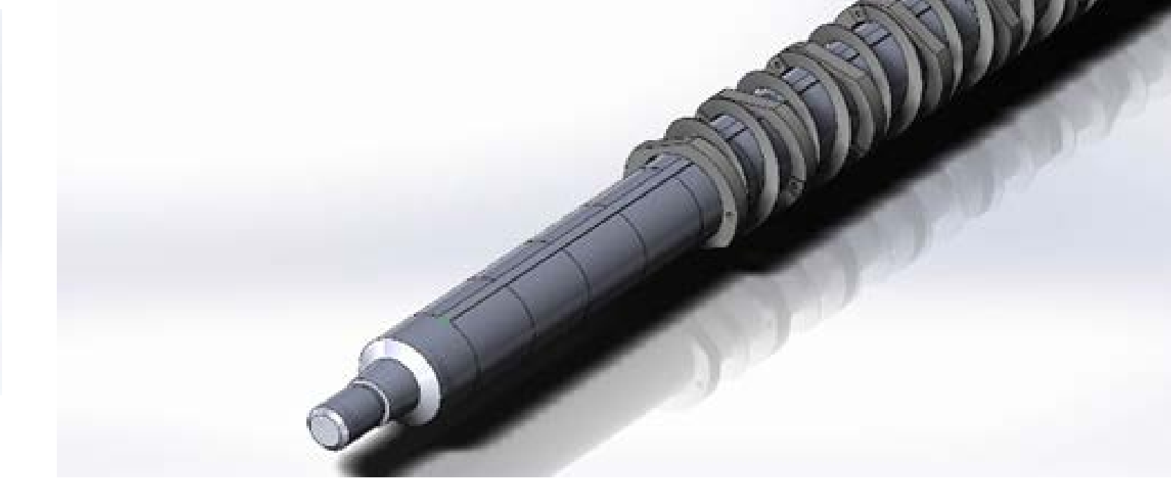
Copper end of current lead. Stacked tapes (except one) are "hidden" to show stepped surface of the copper rod. Double start spiral gas guide can be seen also.
