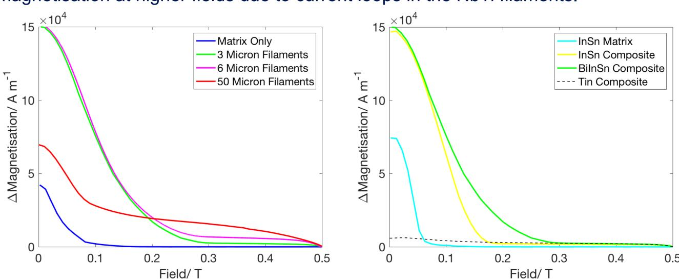
Changing the filament size has limited effect on the critical field for the same loading until filaments become very large. Similar enhancements in higher field performance have been observed with other lead-free solders (InSn), but the matrix must be superconducting to see this effect.
