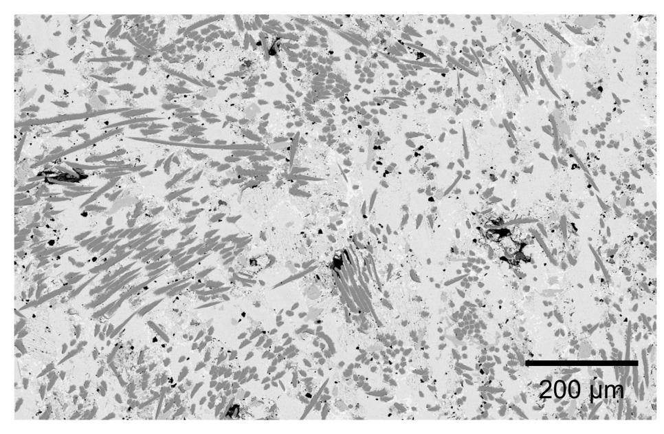
electron microscopy (SEM) of the composite reveals little sign of the original bundle filament structure and good randomisation of the structure. filament There is no evidence preferential nucleation of one of the solder phases onto the NbTi filaments
