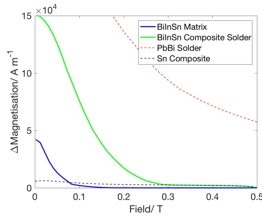
The composite solder demonstrates a significant increase in B<sub>c2</sub> compared to the matrix material. It also demonstrates considerably higher ΔM, indicating higher critical current, but it is still worse than lead-bismuth solders. There is some magnetisation at higher fields due to current loops in the NbTi filaments.
