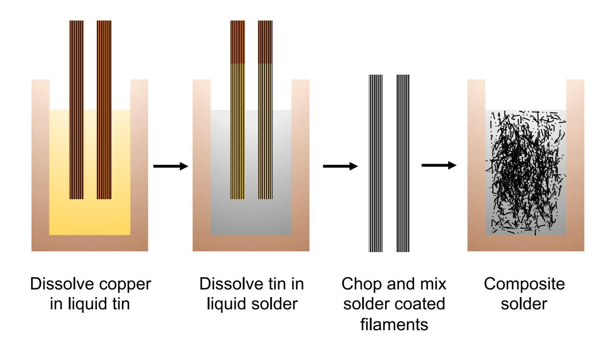
Composite Bi<sub>15</sub>In<sub>50</sub>Sn<sub>35</sub>/NbTi solders are made from NbTi wire containing ~12,000 filaments each 3 µm in diameter. This wire is placed in liquid tin for 90 minutes at 370°C to replace the copper matrix with tin. The tin coated filaments are then placed in liquid Bi<sub>15</sub>In<sub>50</sub>Sn<sub>35</sub> solder at 250°C for 60 minutes to coat them in solder. The wire is then chopped and the pieces melted together and agitated to form the composite solder.
