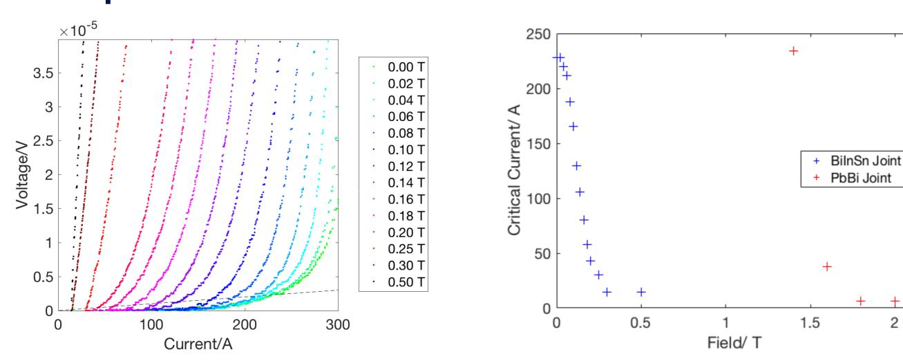
Two 0.5 m sections of multifilamentary NbTi were joined using a solder matrix replacement method<sup>[2]</sup> with Bi<sub>15</sub>In<sub>50</sub>Sn<sub>35</sub> solder. IV curves at different applied magnetic fields were fitted with a 10  $n\Omega$  criteria to determine critical current. A high current was carried at zero field, but the low  $B_{\rm c,2}$  of the solder limited in-field performance.
