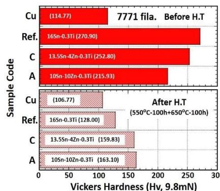
The remained Zn element into the matrix could be acted as the solid solution strengthening factor on the Cu-Sn-Zn ternary matrix after heat treatment.
