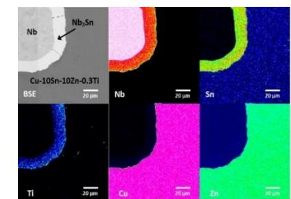
The remained Zn element in the residual bronze will improve the mechanical strength of Nb<sub>3</sub>Sn wire after the heat treatment
