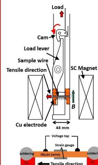
✓ I<sub>c</sub> measurements under unidirectional tensile deformation at 4.2 K and 15T were performed at IMR of Tohoku Univ.
