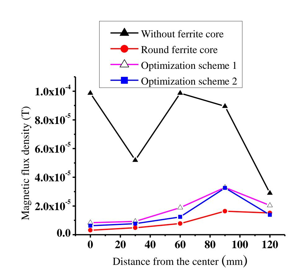
Around the RX-coil, the ferrite cores reduce the magnetic flux density greatly. It means that the ferrite cores can reduce EMI to other circuits.
