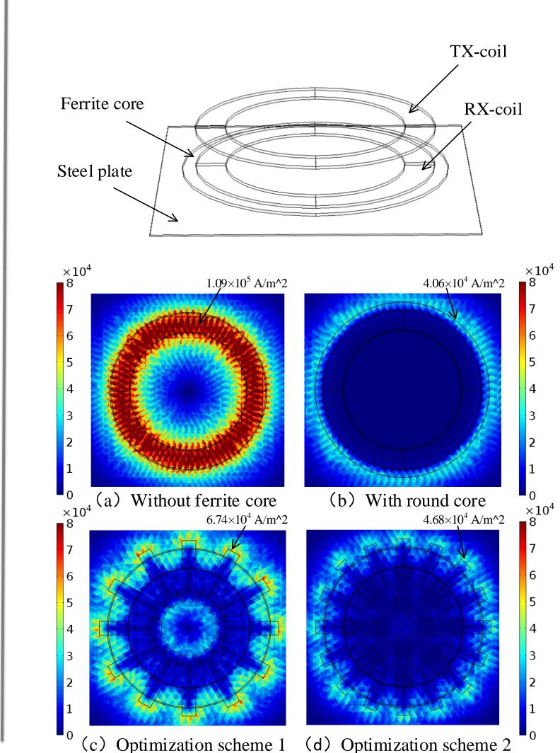
A square steel plate, whose thickness is 1 mm, is placed at a distance of 10 mm from the RX-coil.
