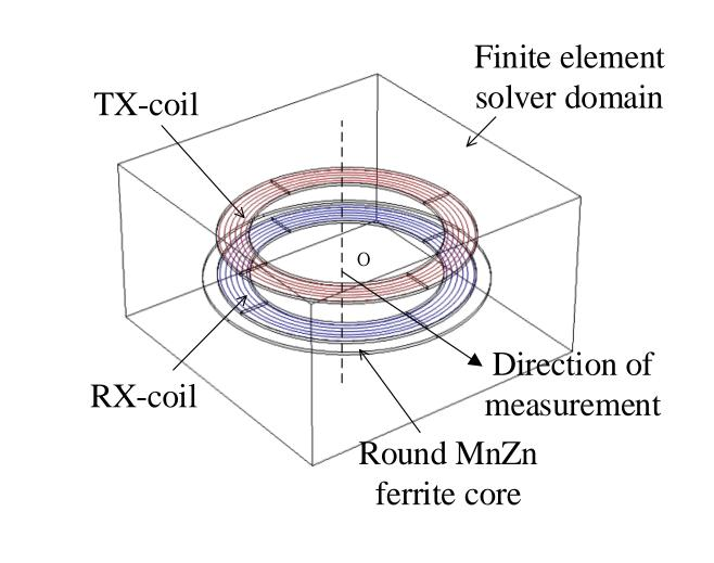
The simulation of the WPT system is carried out with COMSOL Multiphysics. And the system operating frequency is 1MHz.
