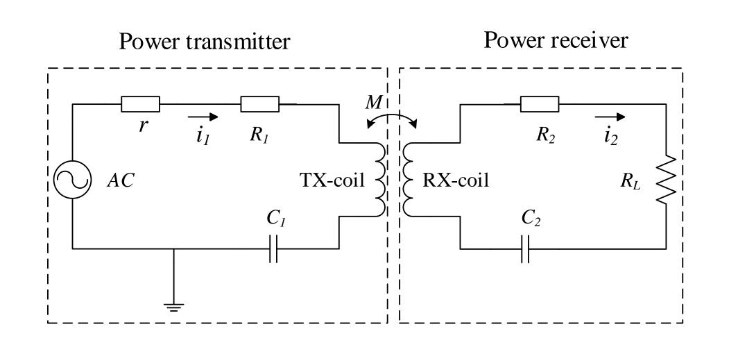
Magnetic resonance coupling is used to transmit power in the WPT system. Power is transmitted through the electromagnetic field produced by the resonant coils (TX-coil and RX-coil).
