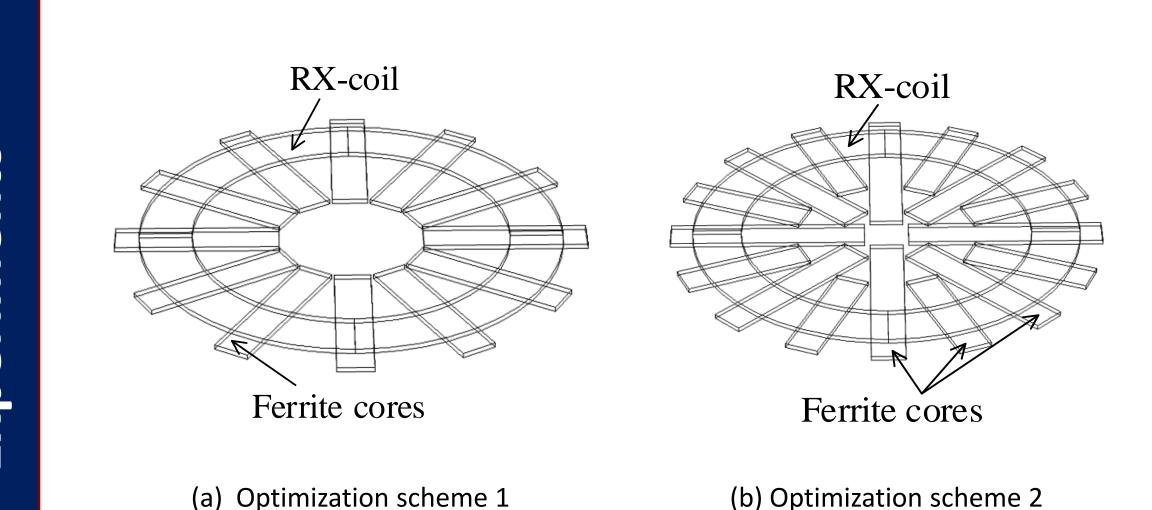
All of the magnetic stripes are made of MnZn ferrite and radially distributed in both of the two optimization schemes. And they are only used in the RX-coil side.
