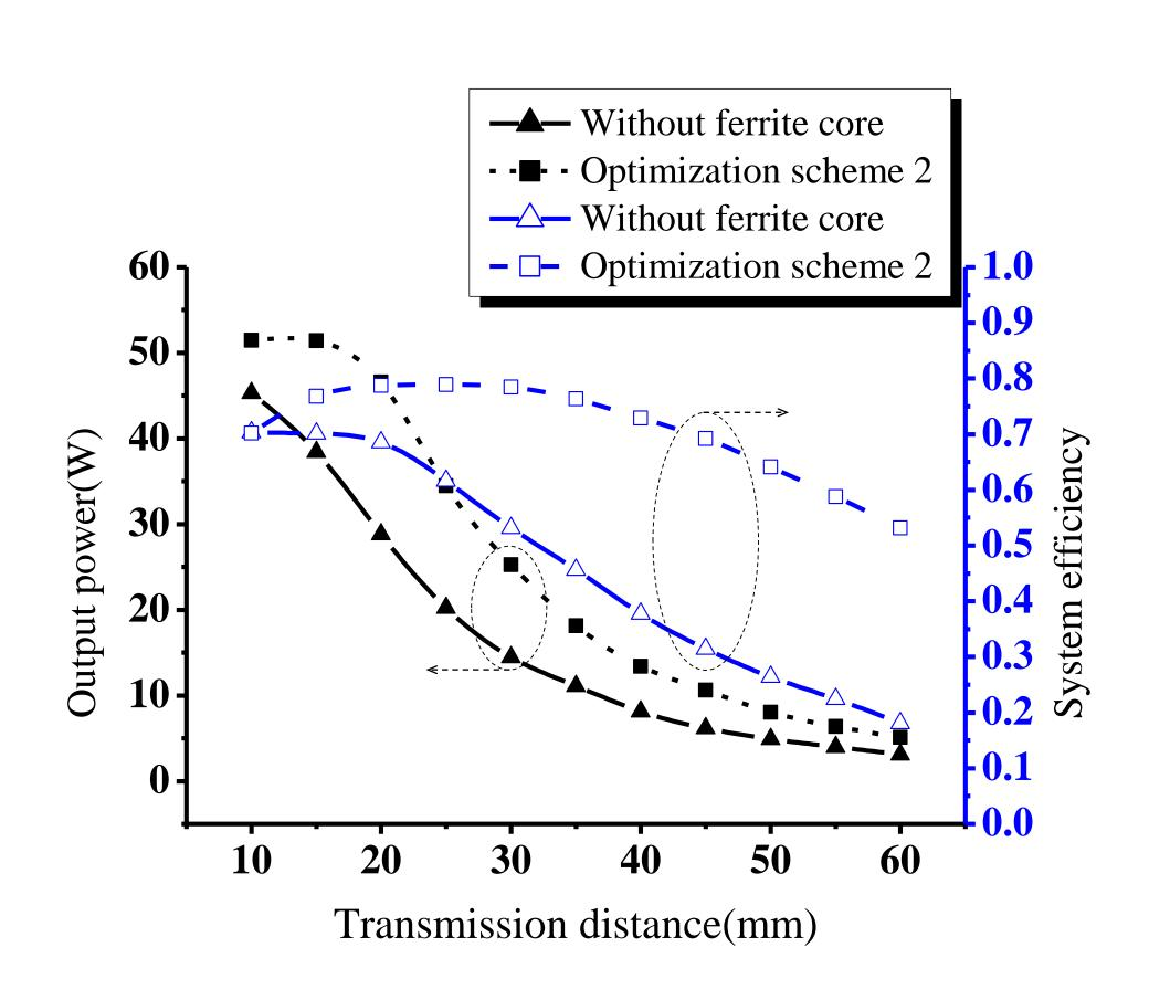
Both of the output power and transfer efficiency are improved when the ferrite core is used. And the maximum improvement in transfer efficiency is 38% at the distance of 45mm.
