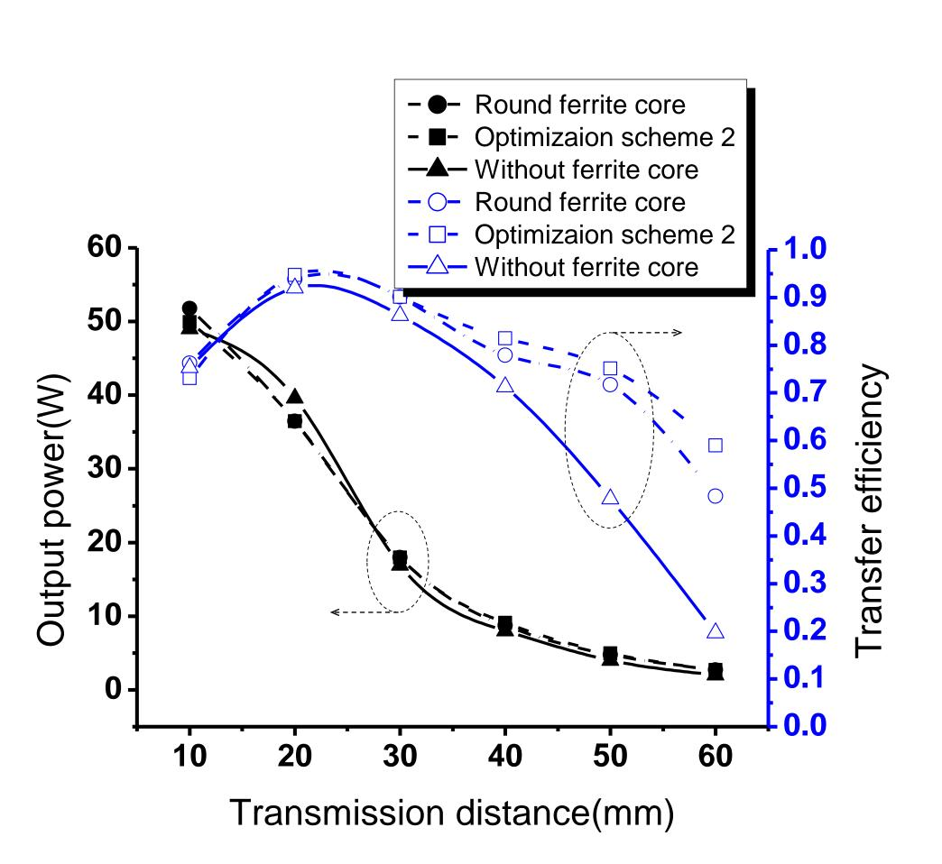
The system with ferrite cores has better performance, especially when the transmission distance is far away.
