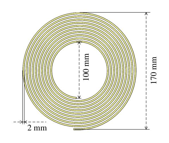
PCB is employed to design the resonant coils of the WPT system to achieve the goal of the smaller size, lighter weight and better integration.
