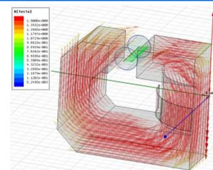
Optimization design of the iron core thickness
