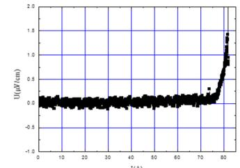
The I-V curve of the prototype YBCO magnet
