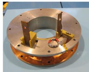
Fabrication of the prototype YBCO magnets.
