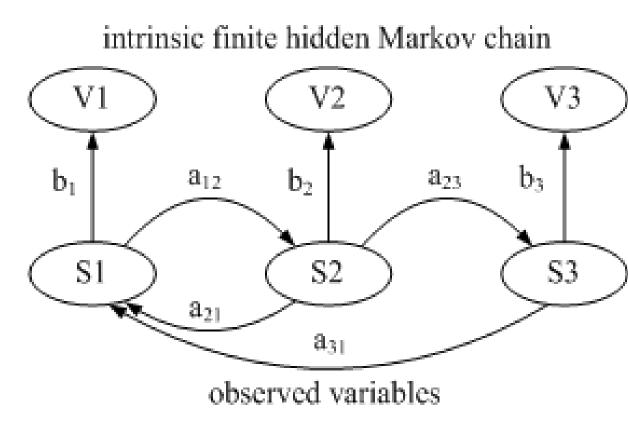
CHMM is a kind of model that describes undetected signals by probability statistics. It is consist of an intrinsic finite hidden Markov and observed variables associated with each state in the Markov chain. These two parts describe signals together and the former one is relayed on the later
