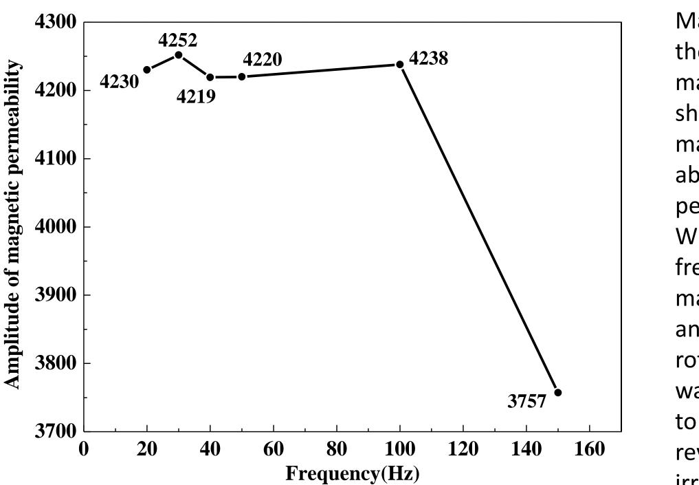
The figure shows the relationship between the amplitude of the magnetic permeability and frequency. It can be seen that the amplitude of magnetic permeability decreases with the increasing of frequency when the intensity of the excitation magnetic field is constant.
