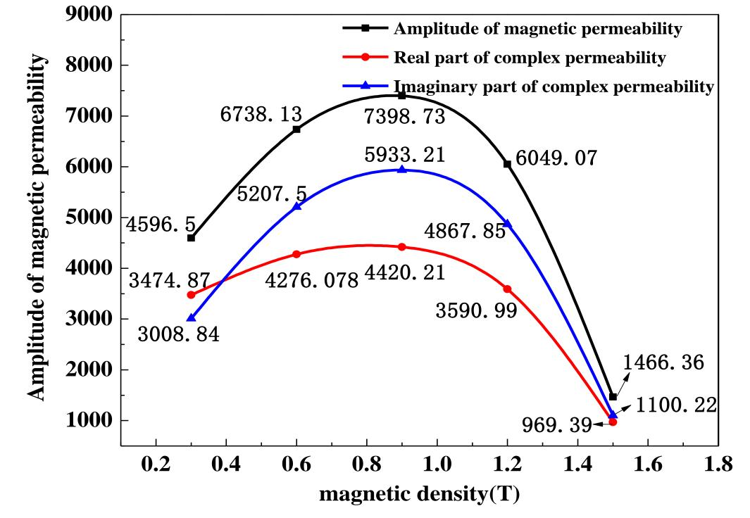
The figure shows the relationship between the amplitude of magnetic permeability and magnetic induction, the real parts of the complex magnetic permeability and magnetic induction, the imaginary parts of the complex magnetic permeability and magnetic induction.
