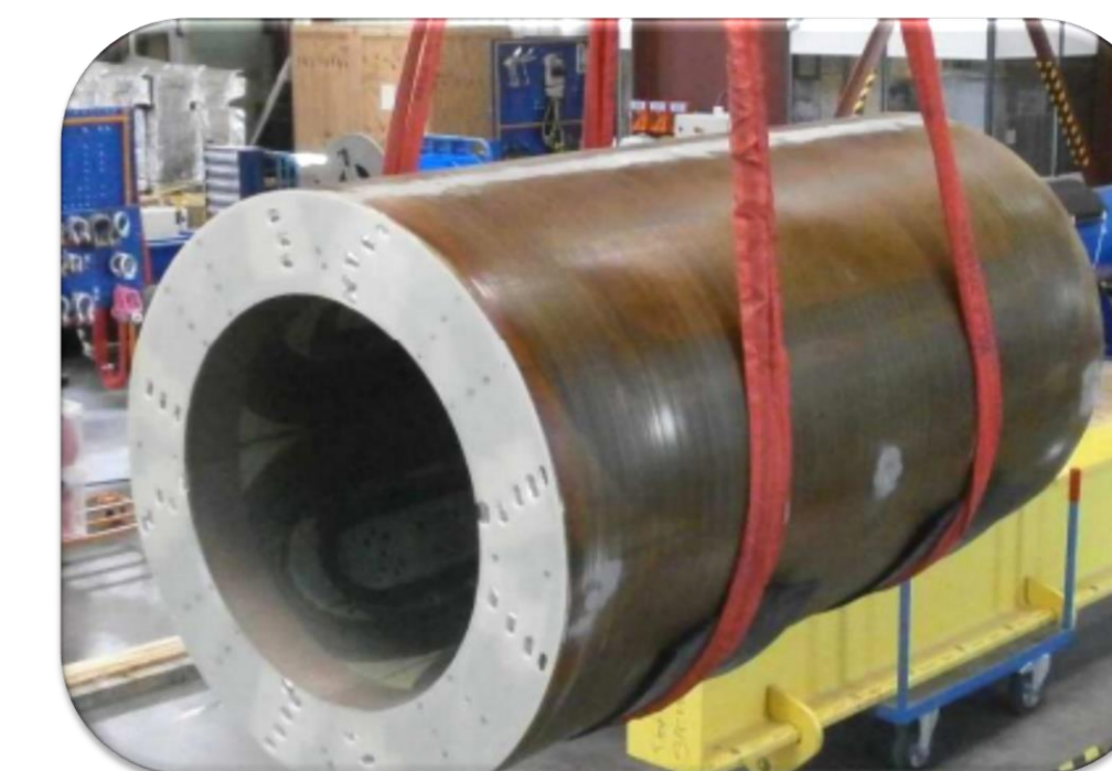
Assembly, ground insulation & final impregnation
