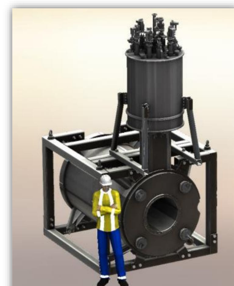
Quadrupole Q2&Q3 - Quantity 2 15 tons Warm bore 600mm Gradient 16 T/m - 4250 A Superconducting NbTi Liquid helium bath
