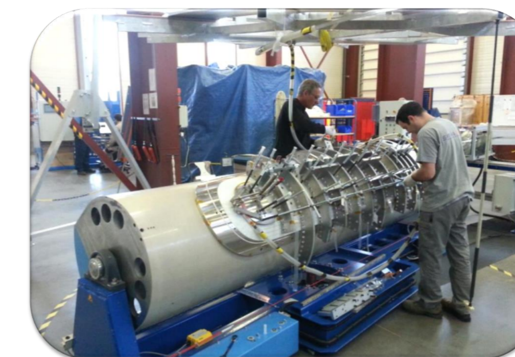
Winding (dipole: 6 layers, Q2/Q3: 8 layers)
