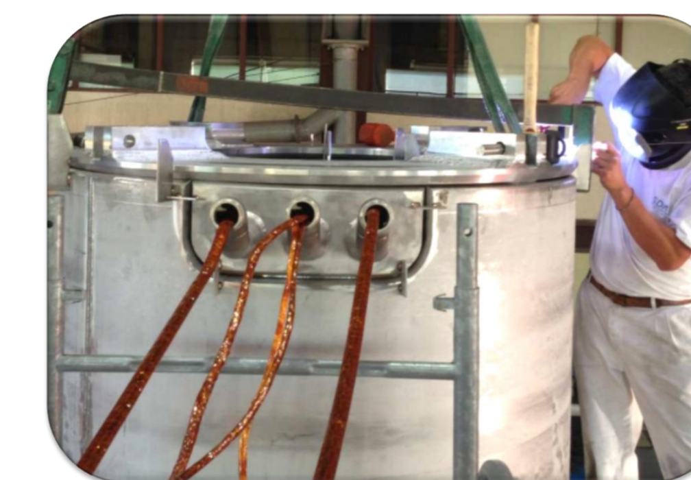
Integration in Helium vessel (ASME welds & controls, pressure & leak tests)
