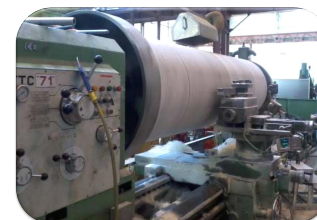
Machining (collars machined after coil OD measurement)
