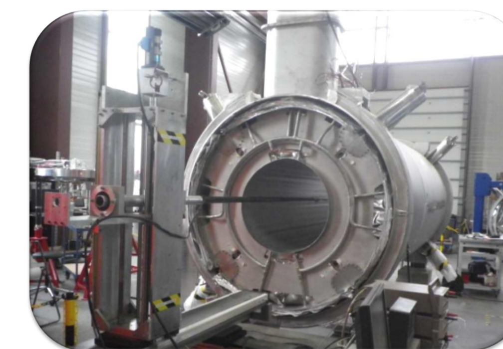
Magnetic measurements with Sigmaphi's mapping table
