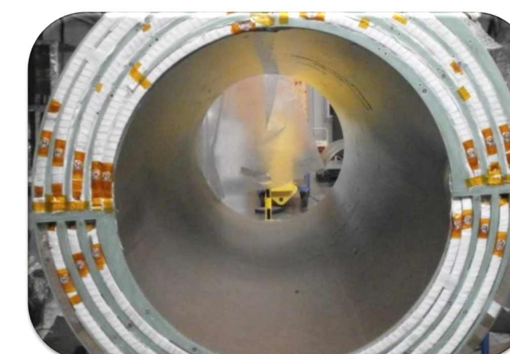
Instrumentation (PT100, Carbon Ceramic sensors & voltage taps)
