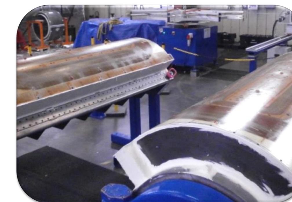
Molding (Resin CTD 101K, a unique molding per pole)
