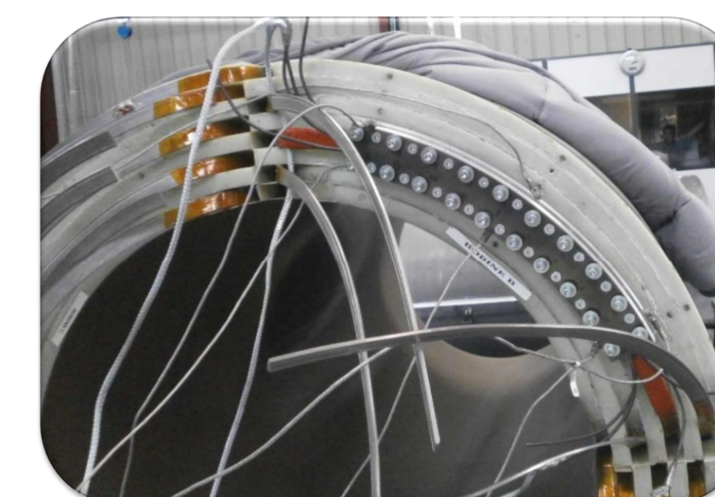
Splicing (process validated with pulling tests)
