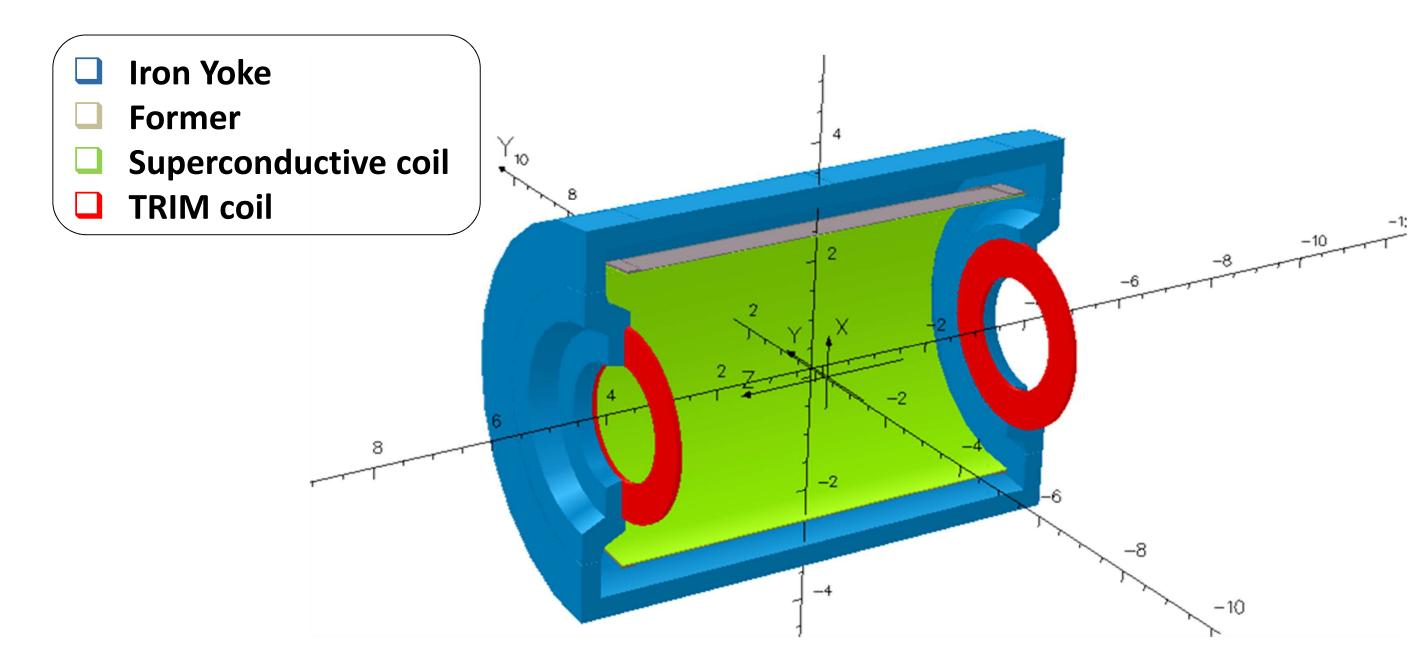
Correction to the main field is provided by two resistive copper coils (TRIM coils) which can be individually tuned in current to reach the requested homogeneity.
