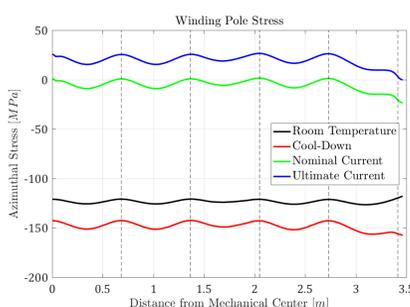
Experiments show that when an insufficient prestress is applied the coil/winding pole/spacers bonding may fail. The consequent motions or even the energy released during the bonding breakage are considered possible quench origins.
