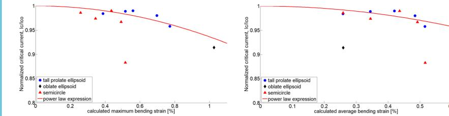
Figures show the normalized critical current according to maximum and average bending strain of tall prolate ellipsoid, oblate ellipsoid and semicircle.
