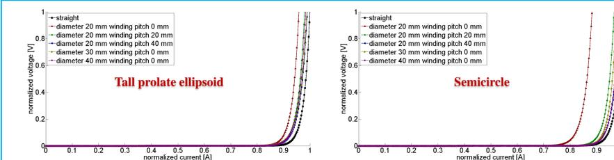
Figures show the normalized voltage according to normalized current of tall prolate ellipsoid and semicircle.
