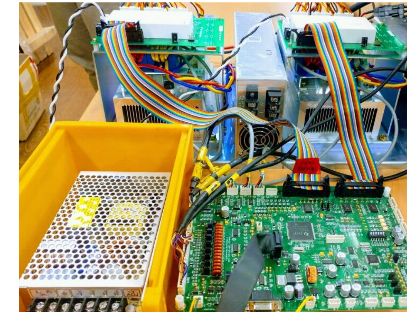
DSP and inverters
