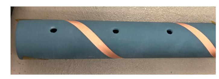
This work investigates the effect of bending on the strain distribution of a tape during circular helical winding, the typical configuration used for the conductor in round core cable (CORC®) [1,2].
