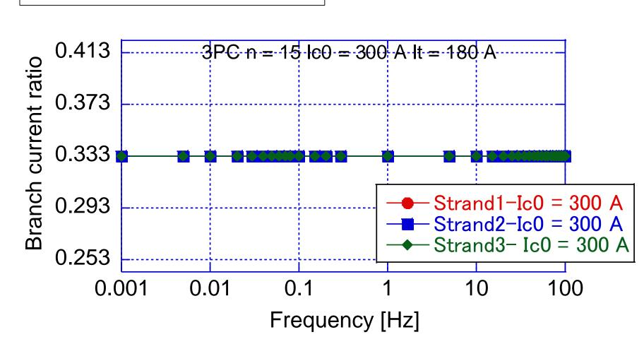
This graph indicates the optimum transposition is performed.
