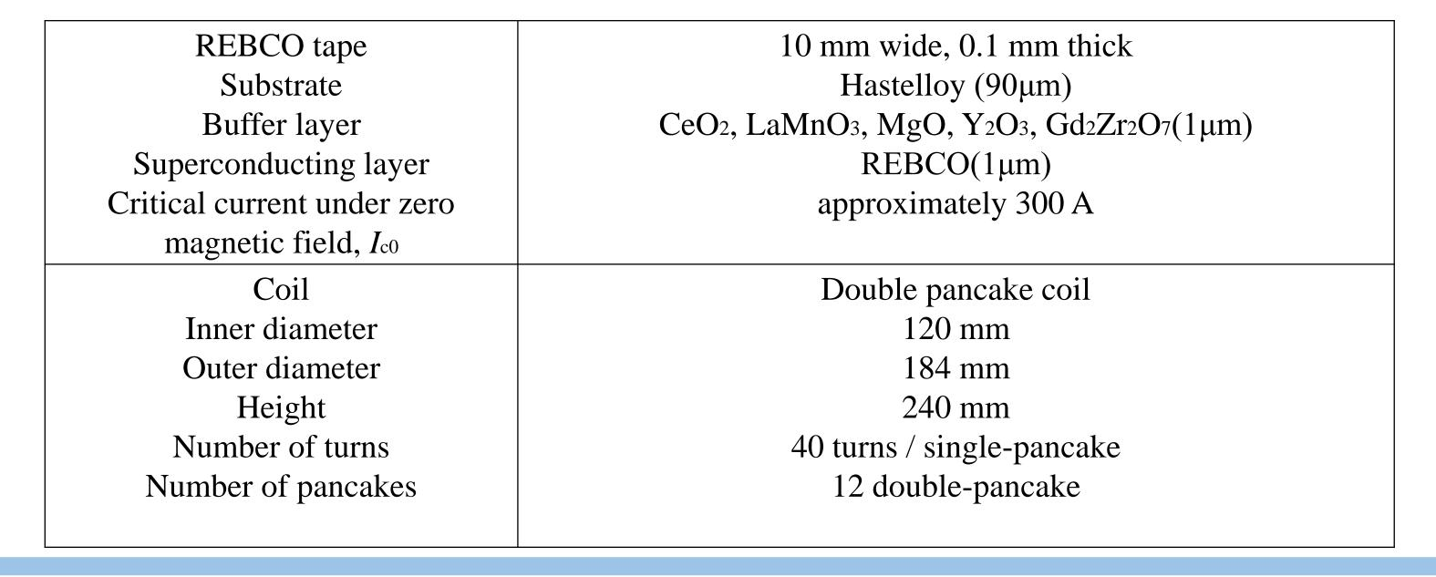
The center magnetic field of the coil is 0.5T Total transport current  $I_t = 180 \text{ A}$
